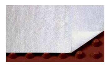
**VersiDrain® 8 Geo** is a dimpled plastic sheet that provides effective drainage and waterproof membrane protection on foundation walls and other underground structures. The integrated non-woven geotextile covering the dimples prevents soil particles blocking the drainage sheet, creates an air gap for reliable ventilation and allows inflow and transport of water from surrounding soil.
