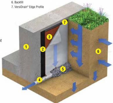
\* VersiDrain® 10 Geo is recommended in situations subject to weight bearing loads of >250 kN/m²
