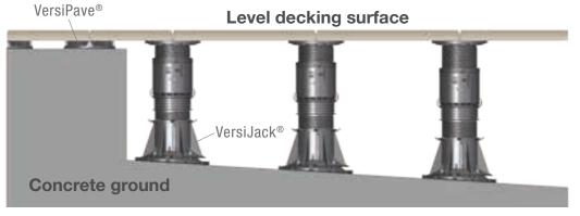
Level decking surface can be achieved by using a combination of pedestals on uneven surfaces.
