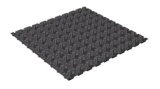
VersiDrain® 25P is a lightweight, water retention sheet used below the growing media that functions to store and drain water and to protect the waterproofing membrane.
