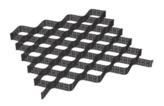
**VersiWeb®** is a cellular confinement system incorporating ultrasonically bonded flexible thermoplastic strips that form a strong, dimensionally stable honeycombed structure which controls erosion by limiting movement of infill within its individual cells.
